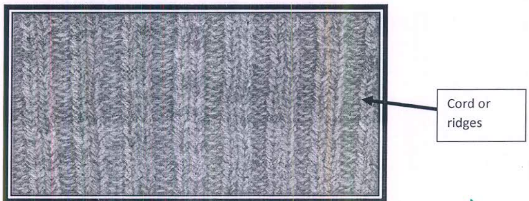
Fig. 2.5: Illustration of technical face Rib knitted Fabric
